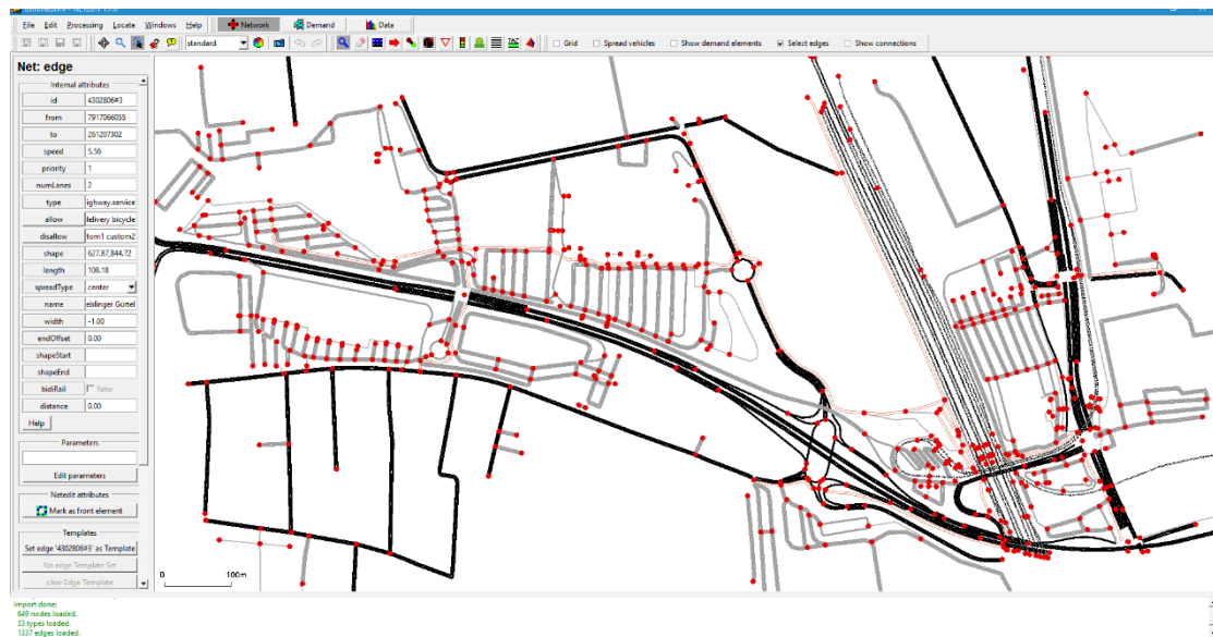
Figure 12: Cleaning up extracted map using NetEdit
